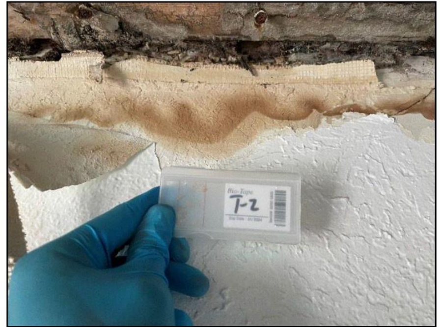
Figure (44) – Surface Mold Sample T-2, collected from the drywall wall in the bedroom of Apartment 6.
