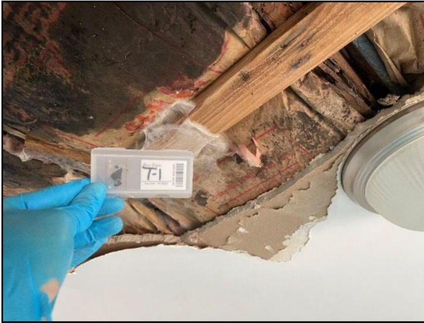
Figure (43) – Surface Mold Sample T-1, collected from the insulation backing above the drywall ceiling in the bedroom of Apartment 6.
